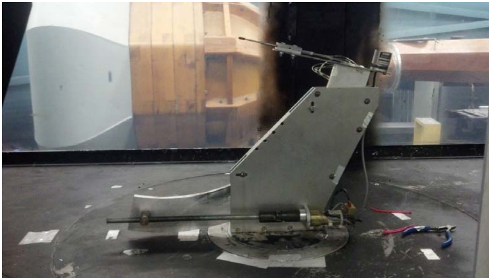
Figure 35 ODU LSWT Pitch Crescent Model Support
