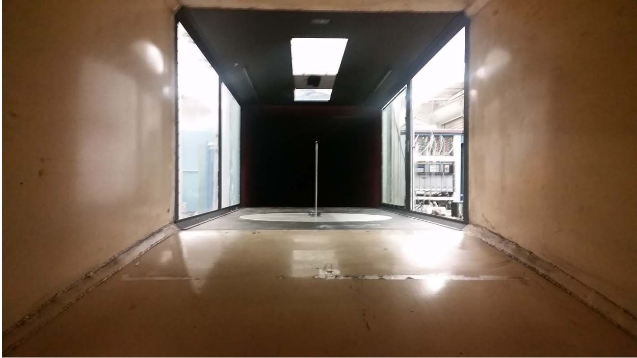
Figure 48 Pitot-Static Tube Installed in the Test Section
