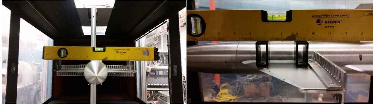
Figure 51 Reference Angle Procedure (Roll Angle Left, Angle of Attack Right)
