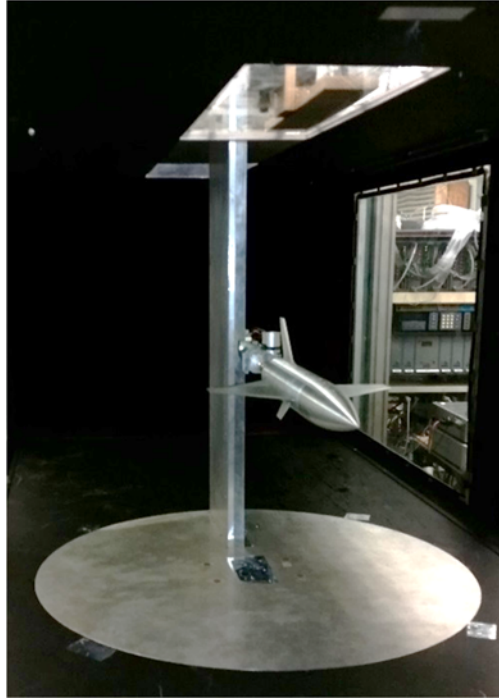
Figure 42 Model Support System Installed in Test Section
